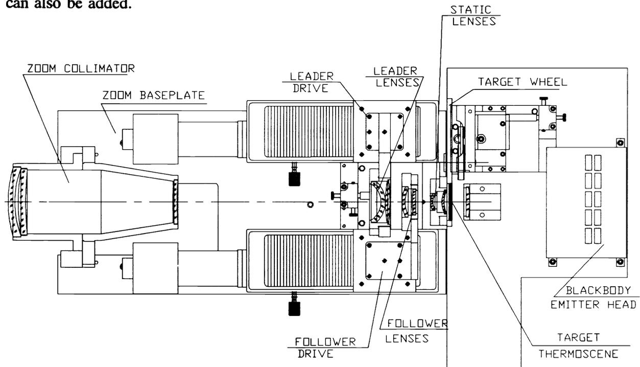
*Figure 7: Typical application of a Thermoscene in a dynamic infrared simulation system.*
