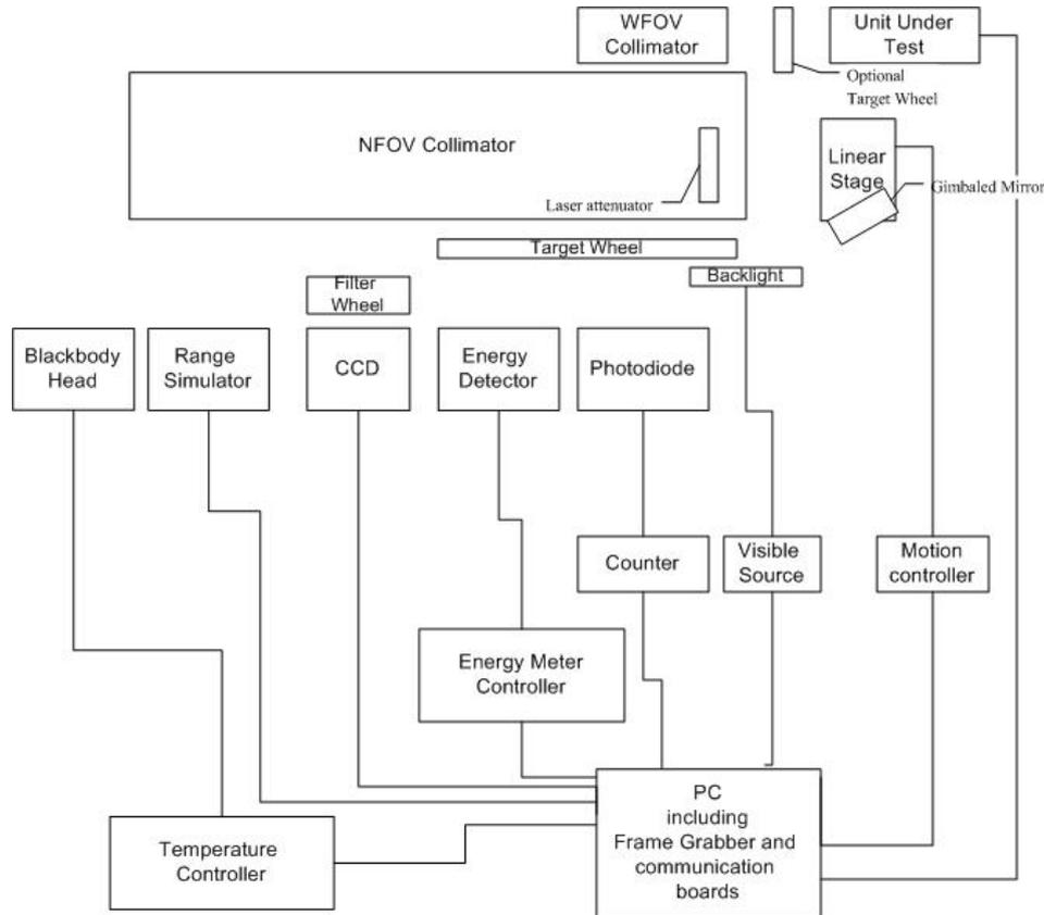
Figure 2: Schematic diagram showing the hardware organization of an EIRT.
